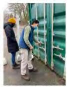
Lift latches which cover the 2 handles on the righthand door.
